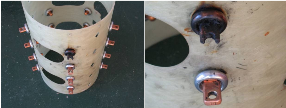
Figure 5: Overheating on the Selector Contact 11.
