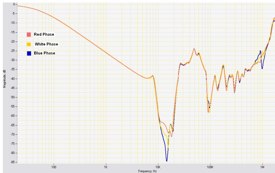
Figure 4: HV Winding to Neutral Short Circuit Response
