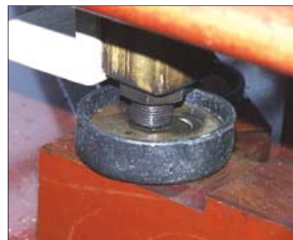
Fig. 5: The source of the PD from winding clamping bolt.
