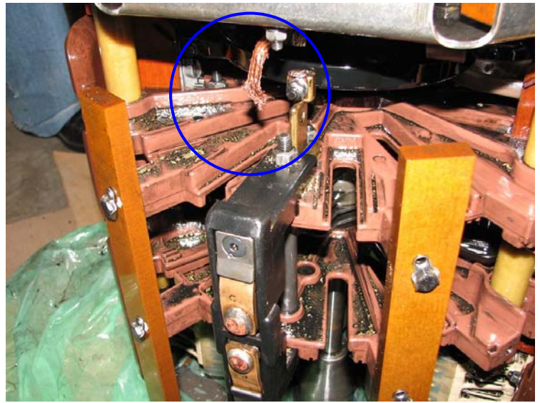
Figure 6: Blue phase diverter- Flexible lead burnt
