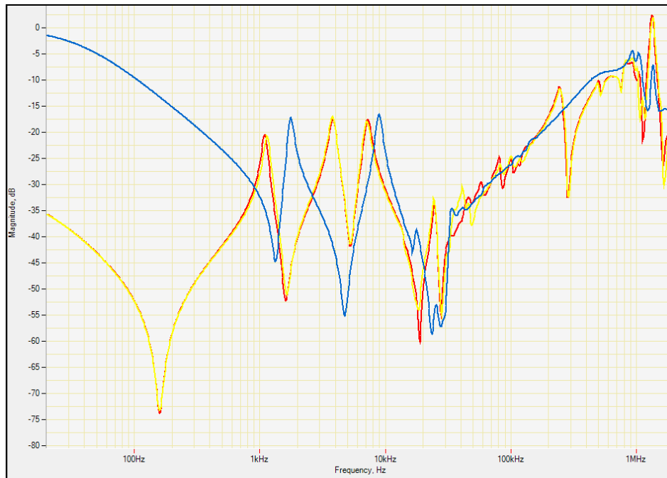
Figure 3: HV to MV winding response
