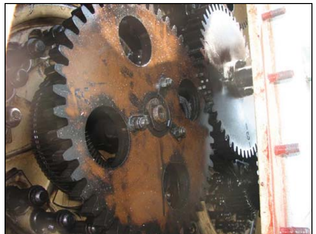
Figure 19: Flashover from Red phase current collector to ground via "insulating" gears.
