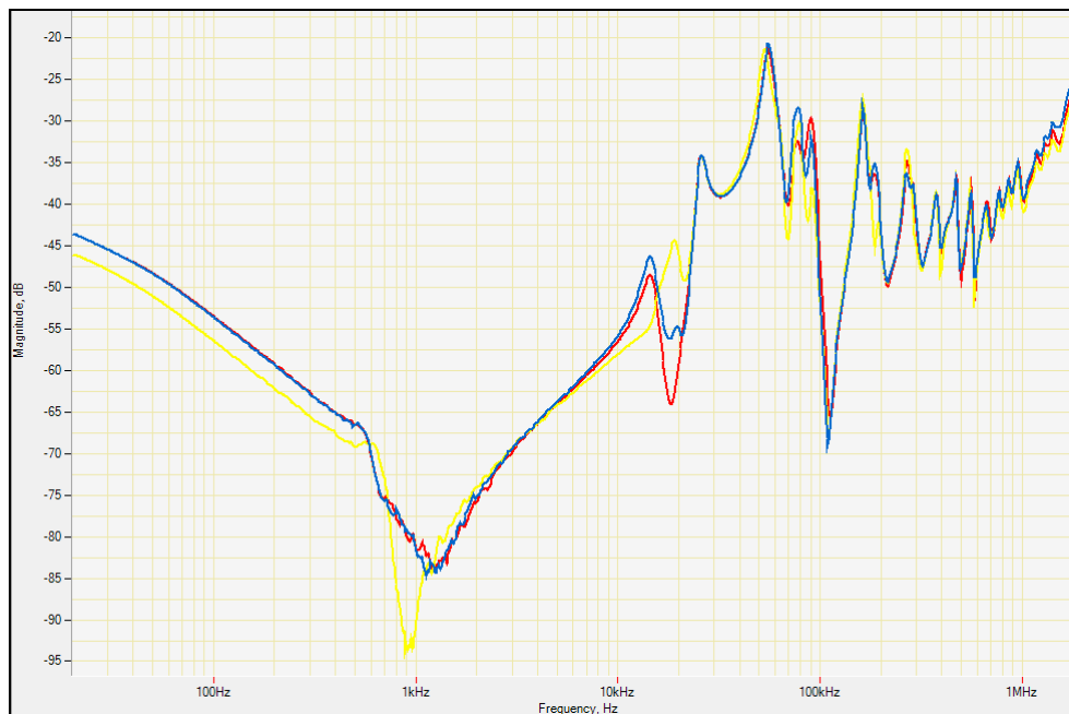
Figure 21: SFRA after repairs to tap changer
