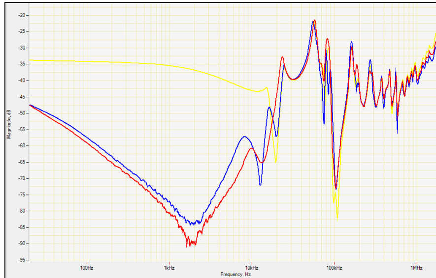
Figure 17: HV to MV winding response
