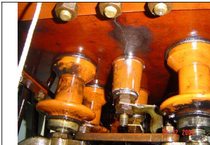
Figure 22: Flashover in diverter- phase to earth fault
