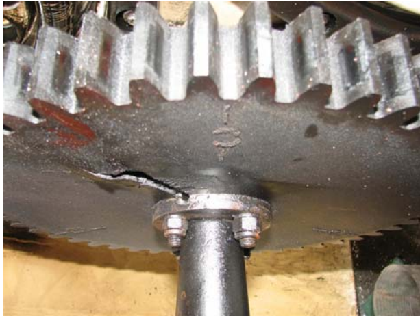
Figure 20: Damaged main gear
