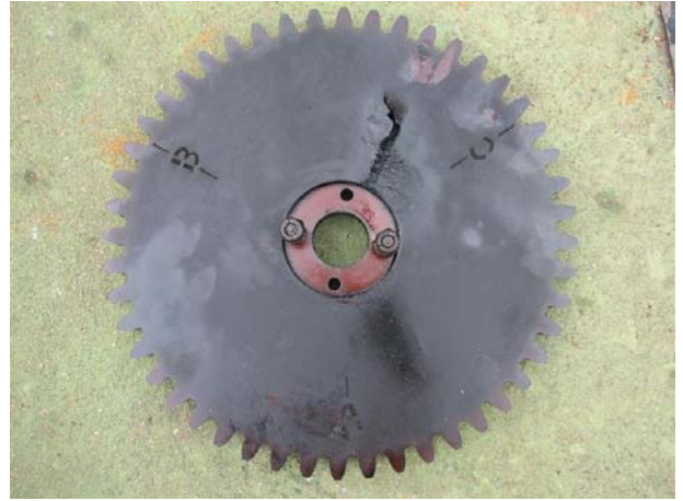
Figure 20: Damaged main gear
