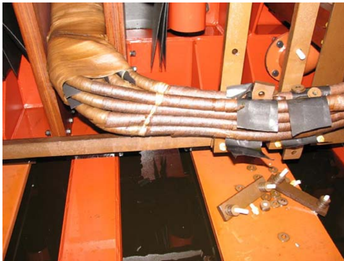
Figure 11: Blue phase tapping leads and broken cleats
